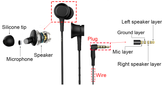
Fig. 4. The components of the earphone.
